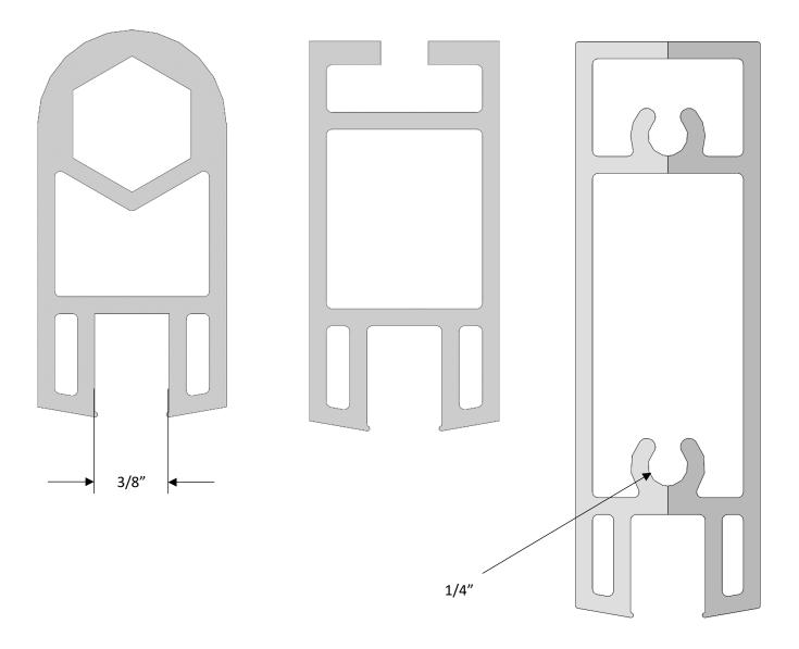
Used From June 2021 – Current 3/8" Glass slot uses these glazing seals:
